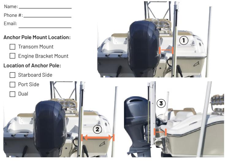
1. Measure from the side of the motor cowling to the anchor. If dual, measure the port and starboard sides.
